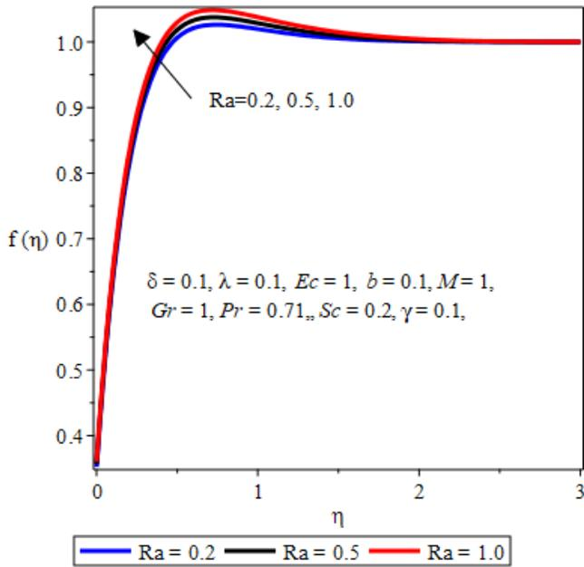
**Fig. 5: Effect of Radiation parameter  $Ra$  on velocity**
