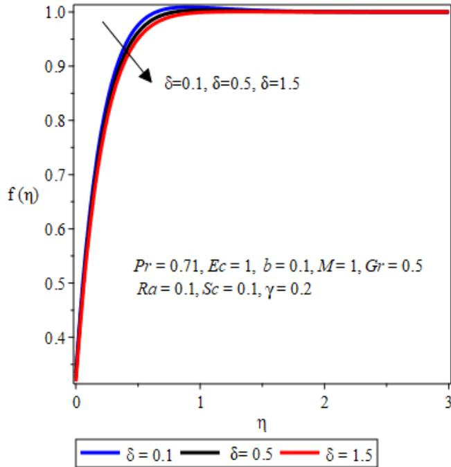
**Fig.10: Effect of temperature jump  $\delta$  on velocity**
