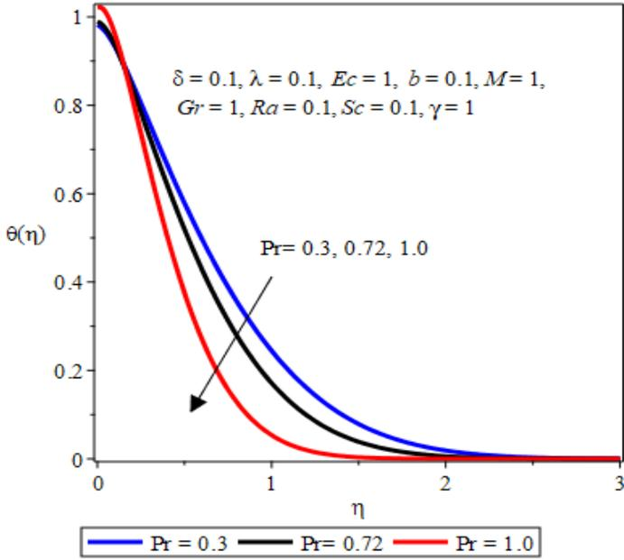
Fig. 15: Effect of Prandtl number Pr on temperature
