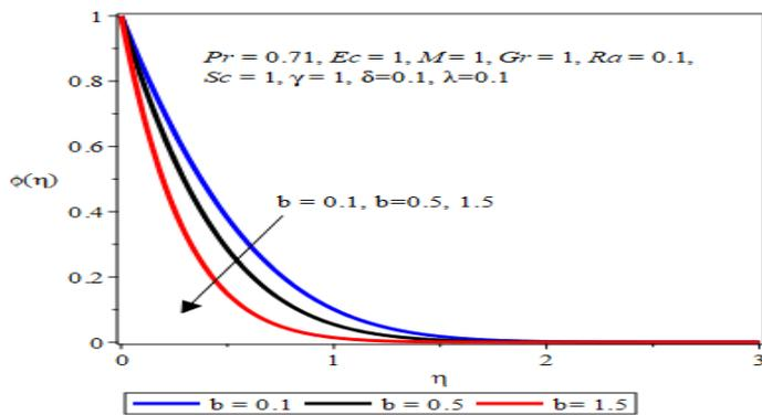
**Fig. 20: Effect of Suction parameter  $b > 0$  on concentration**
