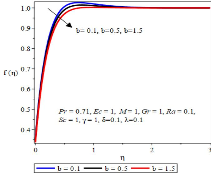
**Fig. 2: Effect of Suction parameter  $b > 0$  on velocity**
