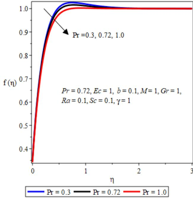
**Fig.6: Effect of Prandtl number  $Pr$  on velocity**
