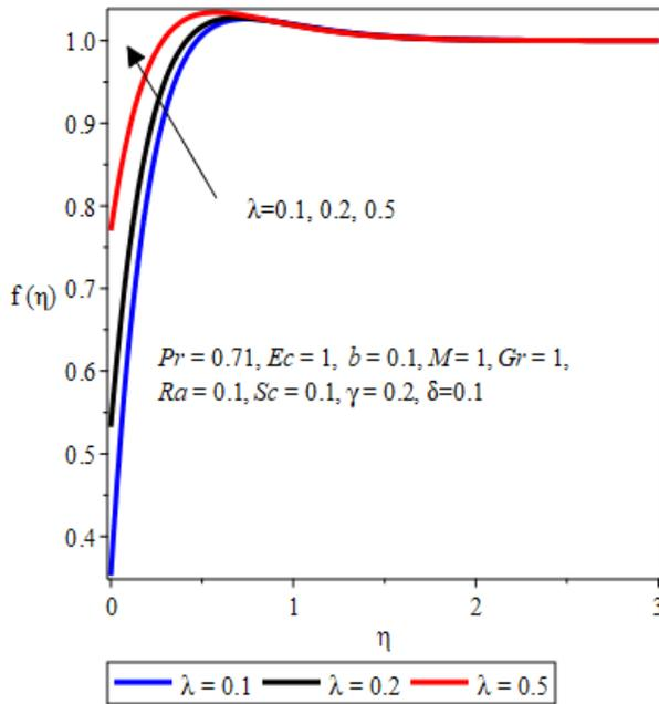
**Fig. 9: Effect of velocity slip parameter  $\lambda$  on velocity**
