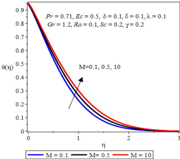
**Fig. 12: Effect of Magnetic field parameter  $M$  on the temperature**
