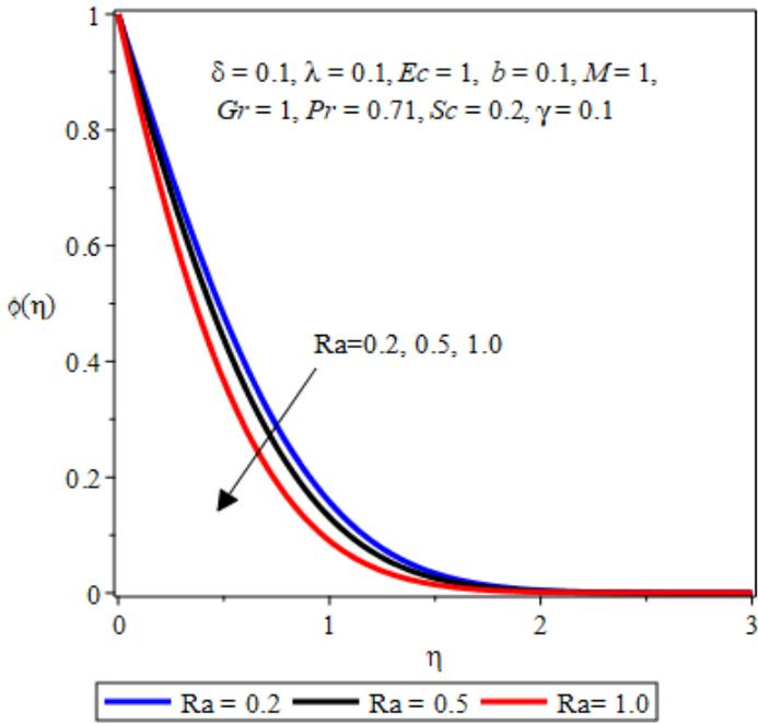
Fig. 22: Effect of radiation parameter Ra on concentration
