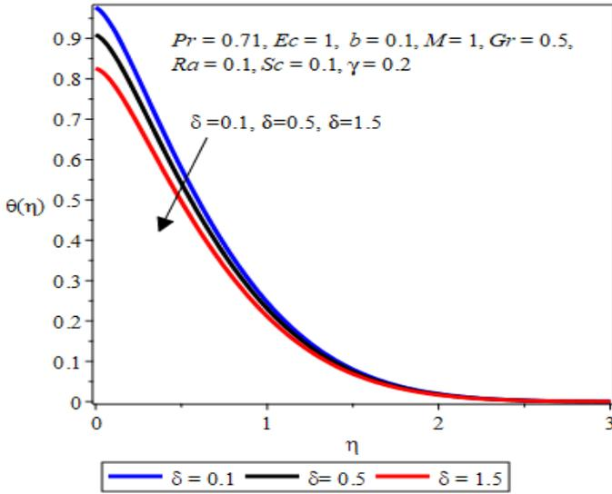
**Fig. 19: Effect of temperature jump parameter  $\delta$  on temperature**
