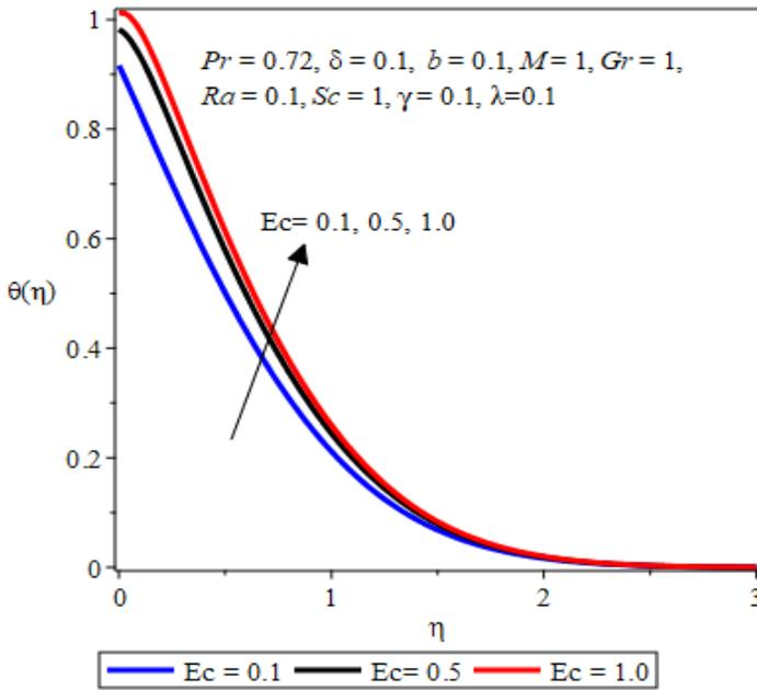
Fig. 16: Effect of Eckert number Ec on temperature
