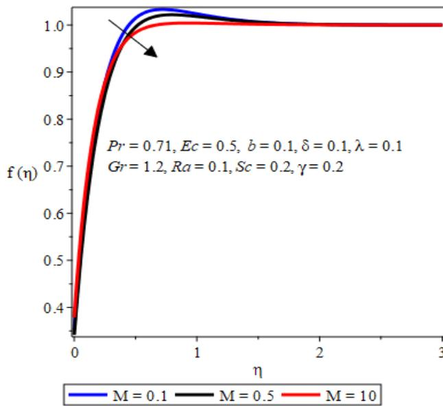
**Fig.3: Effect of Magnetic field parameter M on velocity**
