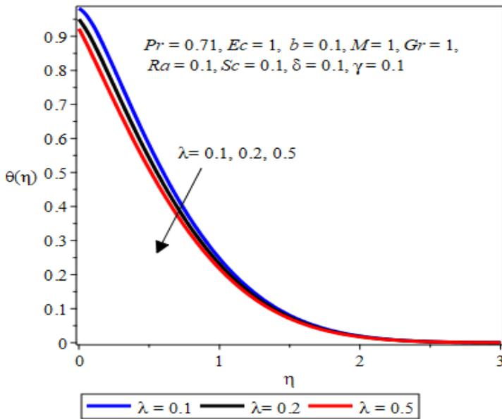
**Fig. 18: Effect of velocity slip parameter  $\lambda$  on temperature**
